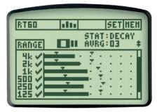
measurement, displaying the RT60 values for a five-octave range (125Hz to 4kHz) as a bar graph and with numerical time values. Multiple measurements can be averaged to provide more consistent results, and the system can also display correlation and uncertainty percentages, which are used to justify the statistical accuracy of RT60 measurements.
